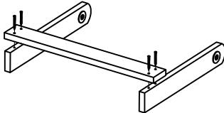
**3)** Attach Back Support Brace (shorter piece) to Back Support Sides with four A screws.
